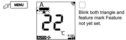
2. Enter Direct Air/Indirect Air set by press MENU button. triangle mark will stop blink and setting feature will be blink instead.
