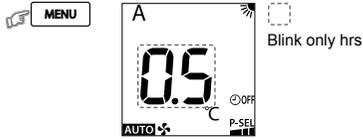
3. Select TIMER OFF by press TEMP. button. Can select TIMER OFF from 0.5 - 12 hrs.
