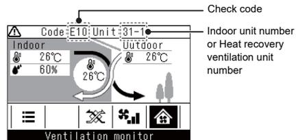
When a trouble occurs in the Heat recovery ventilation unit, the check code and the Heat recovery ventilation unit number flash on the display of the remote controller.
